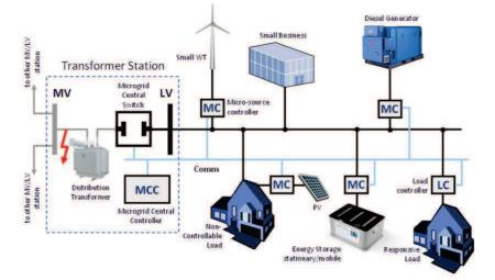
Protection must respond to both utility grid and microgrid faults utility grid faults: protection isolates the microgrid from the utility grid as rapidly as necessary to protect the microgrid loads. microgrid loads. microgrid faults: protection isolates the smallest possible section of the radial feeder to eliminate the fault.
