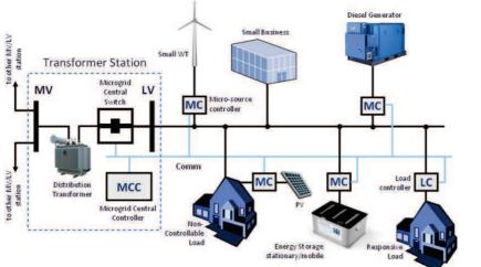
Protection must respond to both utility grid and microgrid faults utility grid faults: protection isolates the microgrid from the utility grid as rapidly as necessarv to protect the microgrid loads. microgrid faults: protection isolates the smallest possible section of the radial feeder to eliminate the fault.
