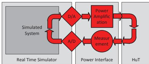
The implementation of PHIL tests environment enforces the use of a dedicated power amplification units (PA).
